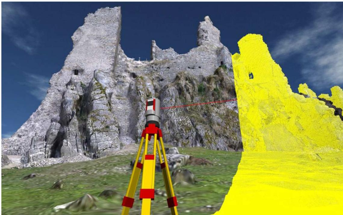
*Figure 1: HELIOS simulating a terrestrial scan of a rock outcrop and castle ruin with a Riegl VZ-400 device. The red line indicates the path of the currently simulated laser beam, the yellow colour indicates the simulated point cloud. (Outcrop & Castle model: CC-BY-NC sketchfab.com)*
